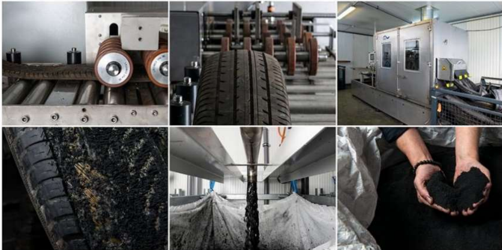
Rubber powder obtained from ELTs recycled with the application of high-pressure water
