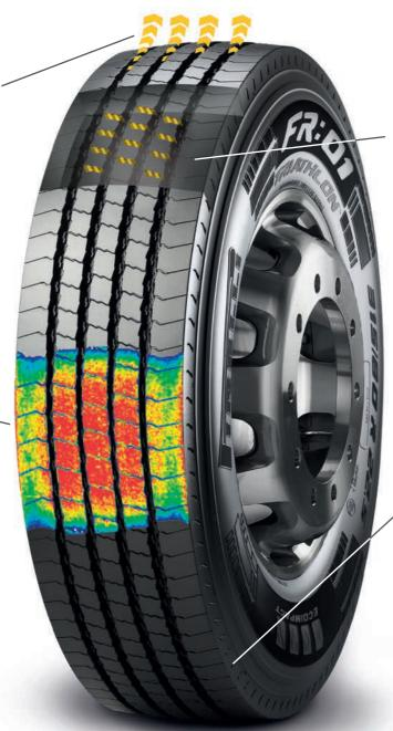
Functional sipes and ejectors at the bottom of all grooves grant superior snow grip, enhance traction and prevent stone trapping
